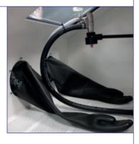
All cabinets have sealed gauntlet gloves, a protected toughened glass viewing window and a quick release media changeover facility.
